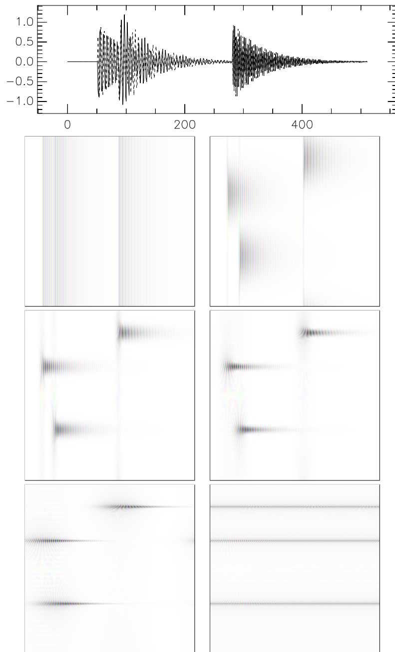
Figure 2.3: GABOR transforms with different window sizes of the complex signal displayed at the top. The result of the GABOR transform contains complex values which are displayed as follows: The darkness of a dot corresponds to the absolute value of the GABOR coefficient and the colour corresponds to the complex argument (the angle or the phase shift). The frequency zero is in the vertical centre. The sign of the frequency corresponds to the orientation of the complex helix. The first image was generated with a discrete GABOR window of size one, the last image with a window which is constant. The first one merely shows the time samples of the signal whereas the last image shows the FOURIER transform when viewed from the side. It can be seen that the more sharp the image is in vertical direction the more blurred is it in the horizontal direction, and vice versa. That is, roughly spoken, the uncertainty principle.
